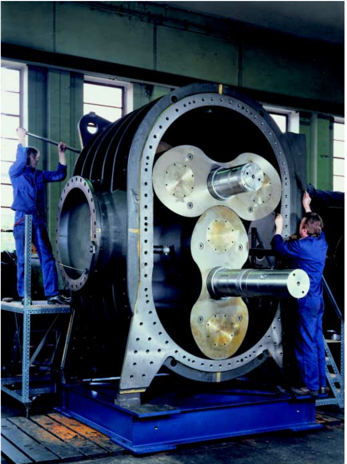
The largest Aerzen Positive Displacement Blower for the oil-free conveying and compression of 65.000 m 3 /h of process gas at an operating pressure of 900 mbar, in a steel plant. Length 3750 mm, width 2400 mm, height 3000 mm, weight 27,2 t.
